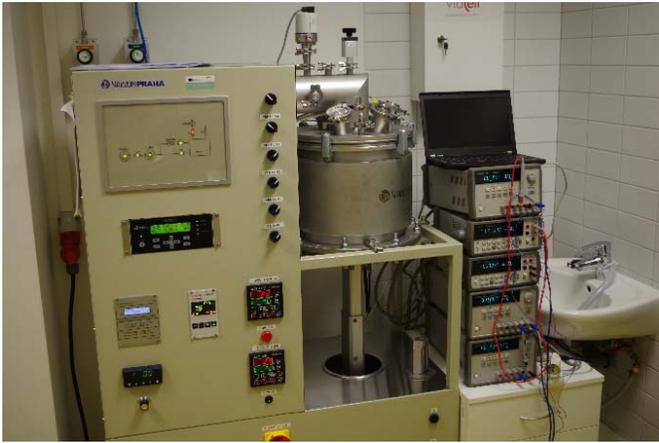
Fig. 2. Vacuum chamber for I-V characteristics measurement.
