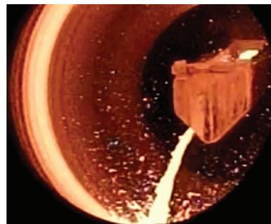
Fig. 4. An early stage of the filling ( $t < 5$  s); a filling jet emitting from the filling arm, splashing on the rotating inner wall of the mold ( $R=0.372$  m,  $\Omega=71.2$  rad/s), and forming a ring around the mold circumference. (Online version in color.)
