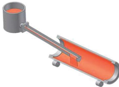
Fig. 1 A schematic of the horizontal centrifugal casting of the outer shell of a work roll
